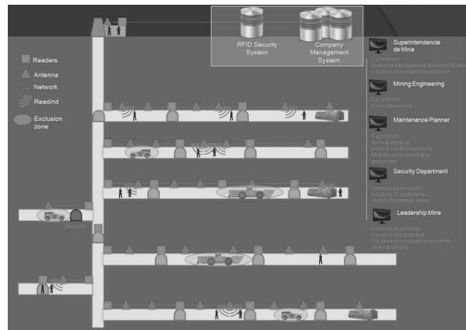
Figure 20.Integral safety system in underground mining.
