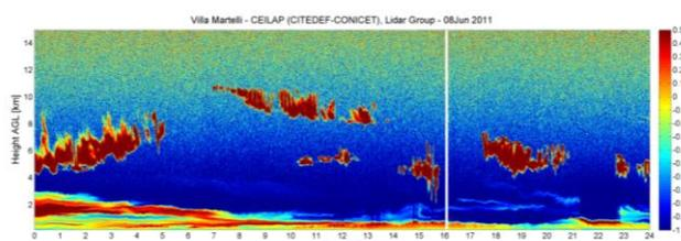
**Figure 3. Aerosol Backscatter at 1064 nm, June 8, 2011.**
