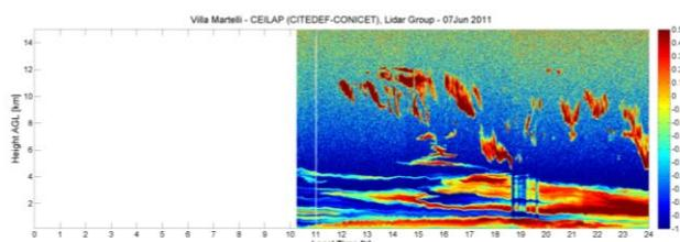
**Figure 2. Aerosol Backscatter at 1064 nm, June 7, 2011.**
