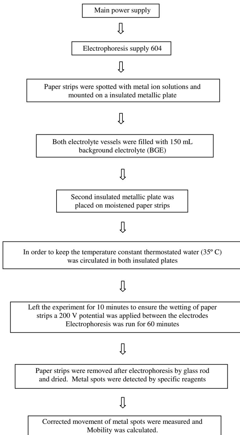
**Fig. 3** The scheme for paper electrophoresis set-up
